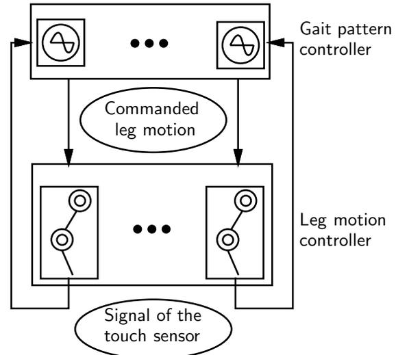
Fig. 2: Architecture of the proposed controller
