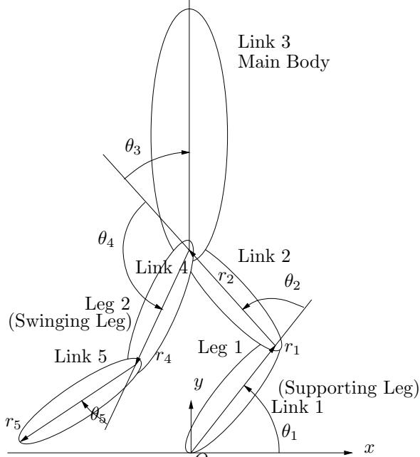
Fig. 1 Schematic Model of a Biped Locomotion
