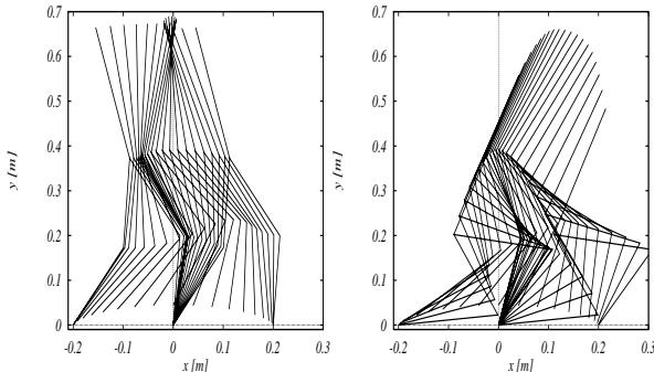
**Fig. 4** Stick figure of a biped locomotion machine
