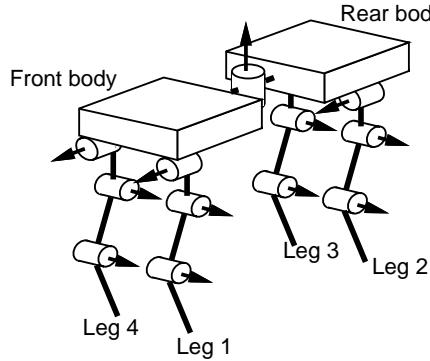
Fig. 1. Schematic model of a quadruped robot
