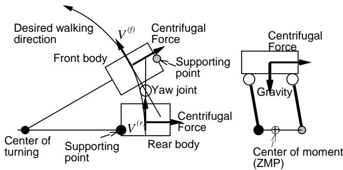
Fig. 4. Dynamic property of turning motion
