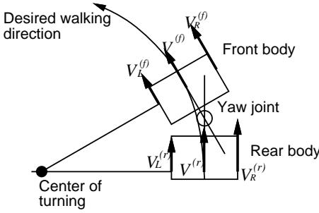
Fig. 3. Kinematics of turning motion
