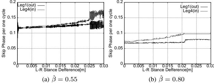
Fig. 5. Reset values of oscillator phase.(Front legs)
