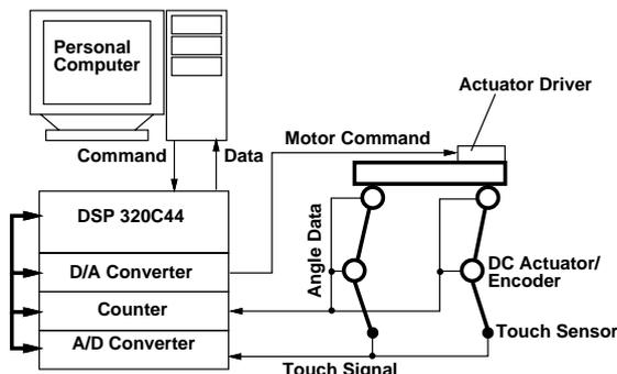
Fig. 12: The data processing system
