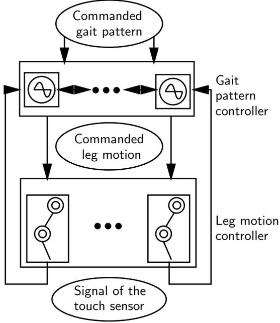
Fig. 2: Architecture of the control system
