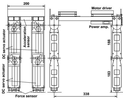
Fig. 11: The mechanical system
