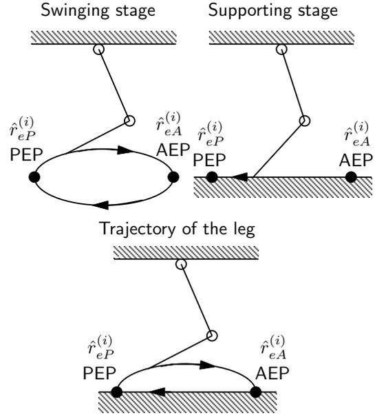
Fig. 3 Trajectory of the leg
