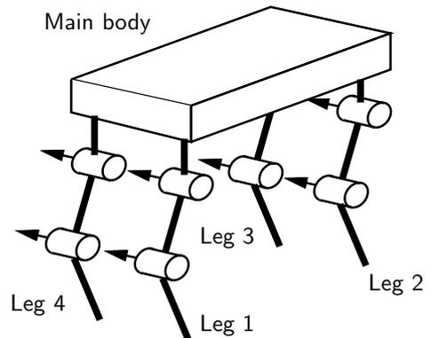
Fig. 1 Schematic model of a quadruped robot
