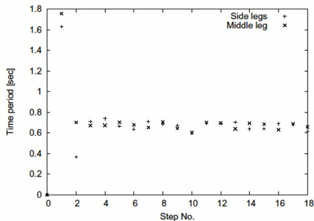
Figure 8. Walking cycle time for each leg
