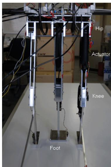
Figure 6. Robot hardware
