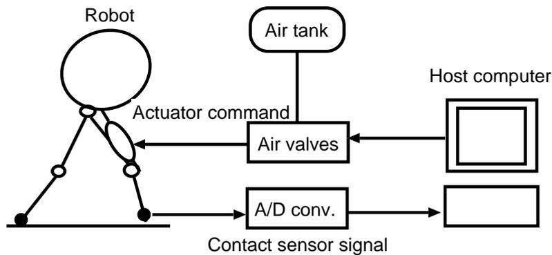
Figure 7. Architecture of hardware setup
