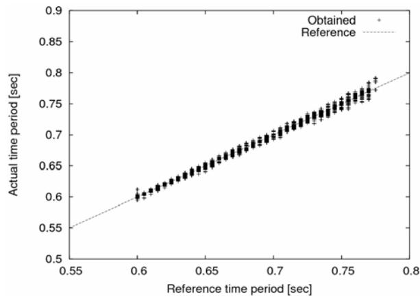
Figure 5. Walking cycle time at variable reference
