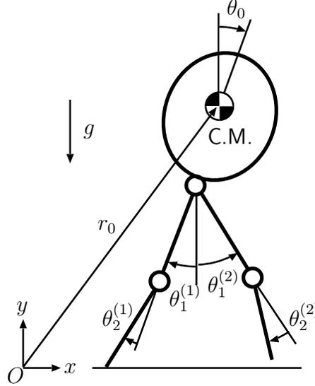
Figure 1. Schematic model of a bipedal robot
