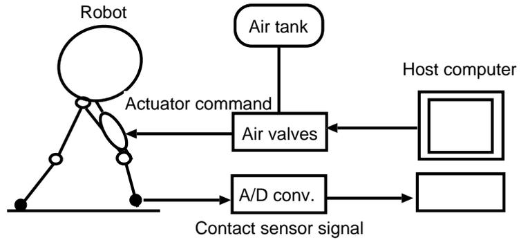
Figure 5. Architecture of the hardware setup
