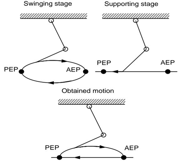
Figure 2: Trajectory of the leg
