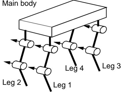
Figure 1: Schematic model of a quadruped robot
